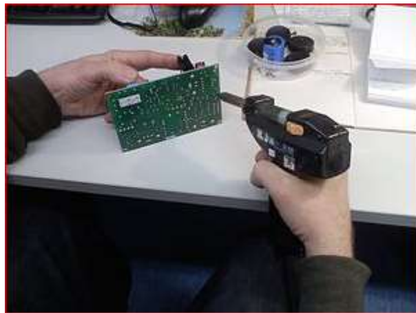
Fig:-6 De-soldering with gun
