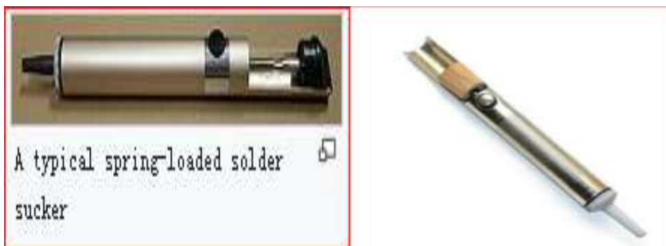
Fig: -7 De-soldering with Solder Sucker
